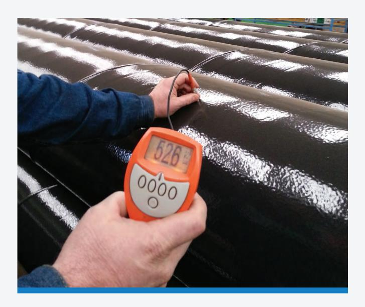
Coating Appearance: Coated steel pipes are visually inspected to detect flaws, such as bubbles, cracks, wrinkles, voids, blisters, pinholes and any contamination.
